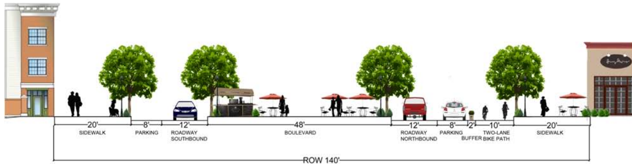
Figure 29: Boulevard Design Option #1 for Ocean Avenue, Sea Bright, NJ Source: Brittany Ashman
