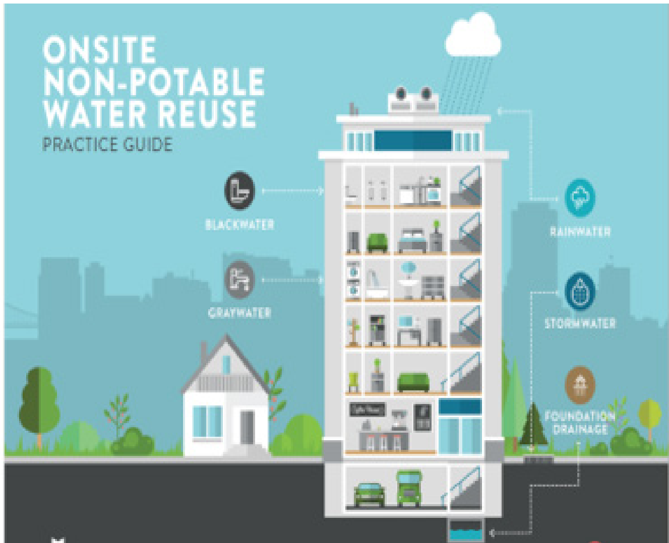
Fig.62. A diagram of residential non-potable water reuse Credit: William J. Worthen Foundation
