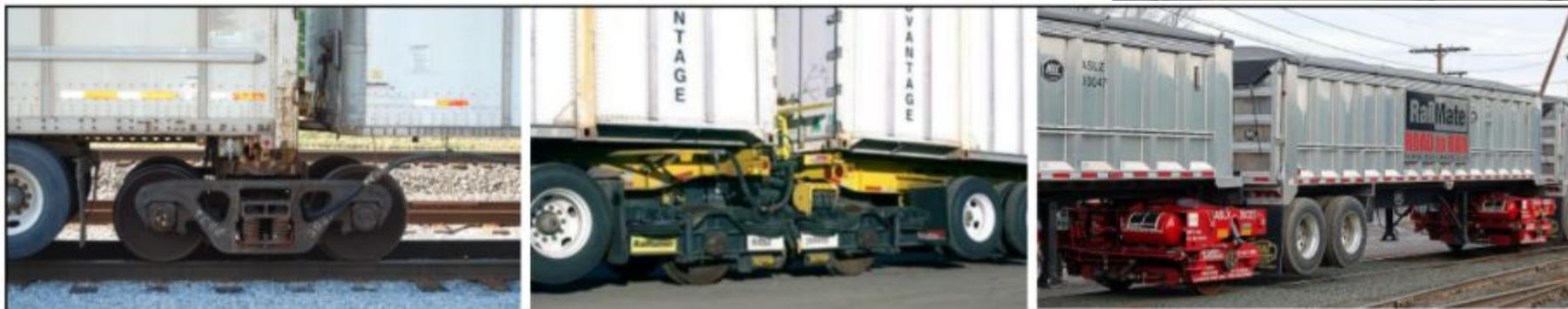
Versions of carless technology by three manufacturers. (Left to right: RoadRailer, RailRunner and RailMate)<sup>3</sup>
