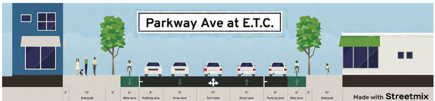
Figure 10: Proposed design for Parkway Ave at Ewing Town Center. Similar to the existing proposed Parkway Ave Enhanced Road Diet designs (“Concept Plan” 2019), these modified designs incorporate class IV bike lanes protected by parking.
